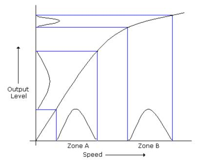
You will observe that speed variation around level B has very little effect on the output variation as compared to the same speed variation around level A. The setting of the contributing parameter of speed to level B therefore makes the process more robust to process parameter variation.
