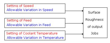
An example of a Machining Process
