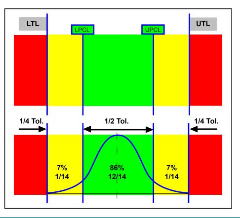
If Cpk of the process is 1.0, it means that the tolerance equals 6x Sigma and the mean of the process coincides with the tolerance mean. Sigma is the standard deviation. In such a cases and assuming normal distribution, we can expect that 86 % of the readings will be in the green (PC) zone and 7% in each of the yellow zones. Thus we can expect one out of 14 readings in yellow zone.
